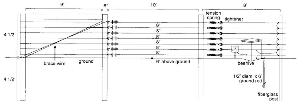
Figure 2: Spacing of wires and gate, and location of beehive, solar panel and grounding rod behind the fence.
