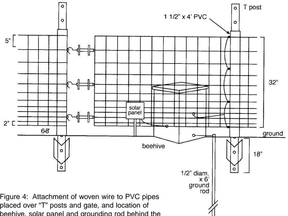
Figure 4: Attachment of woven wire to PVC pipes placed over "T" posts and gate, and location of beehive, solar panel and grounding rod behind the fence.
